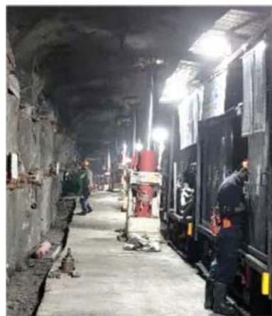
图30 石拉乌素矿辅运巷小煤柱沿空巷道 Fig.30 Gob-side entry with small coal pillar in auxiliary transportation roadway in Shilawusu Coal Mine
