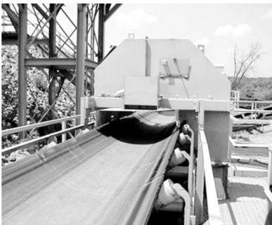
图 1 江比郎公司生产的输送带中部采样装置 Fig.1 Sampling device for the middle of the belt produced by Ebirou Company
