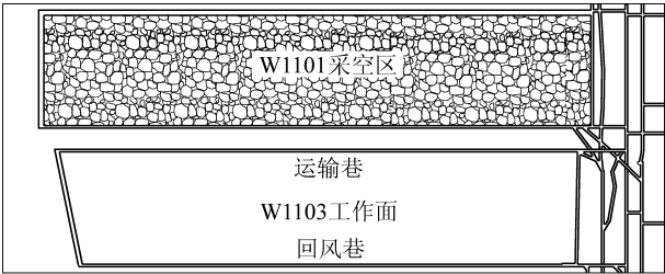
图 8 W1103 工作面布置 Fig.8 Layout of No.W1103 working face
