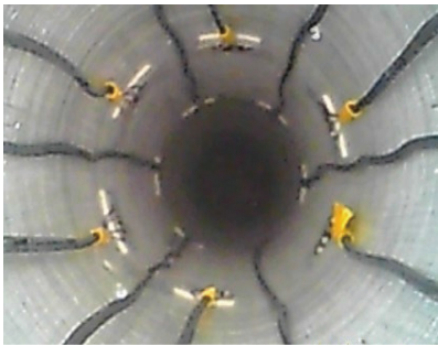
图 3 衬砌模型内壁应变计布置 Fig.3 Diagram of strain gauges on model lining inner wall
