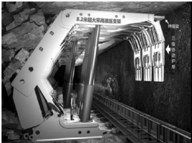
图4 超大采高液压支架伸缩梁与三级协同护帮结构 Fig.4 Structure of extensible canopy and three-stage co-movement face guard for ultra large mining height hydraulic support
