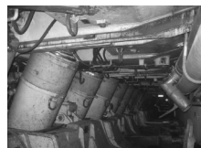
图2 31201综采工作面压架示意 Fig. 2 Support crushing accident of No. 31201 fully-mechanized coal mining face
