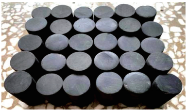
图 1 切割、打磨后的油页岩试样 Fig.1 Oil shale sample after cutting and grinding
