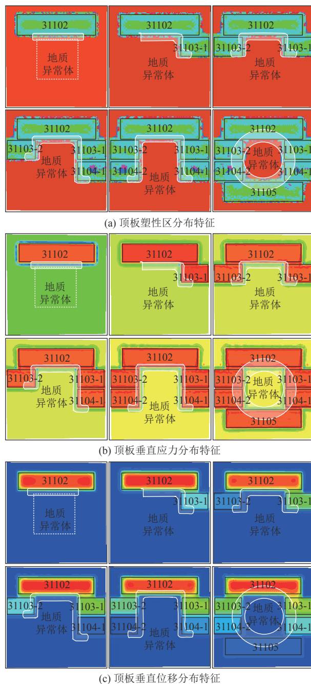
图8 覆岩空间结构演化规律数值模拟 Fig.8 Numerical simulation of overburden spatial structure evolution law
