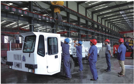
图 29 防爆电动无轨胶轮运输车 Fig.29 Explosion-proof electric trackless rubber wheel transporter
