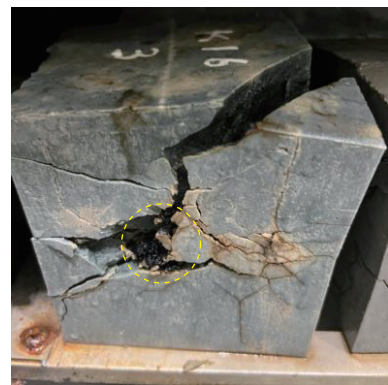
图4 PCCB 试样在成型和养护的过程中发生开裂和破坏 Fig.4 Cracking and failure of PCCB samples occurred during molding and curing
