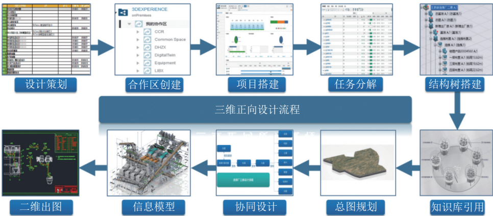
图 3 选煤厂三维正向设计流程 Fig.3 Forward design process of coal preparation plant
