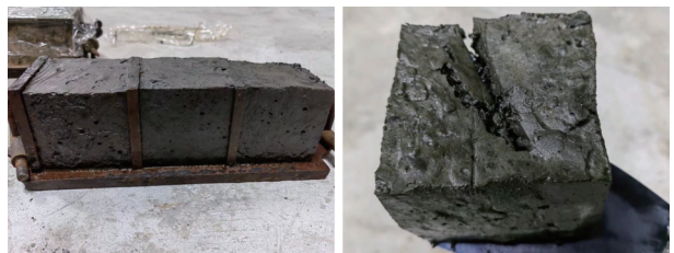
图 10 生物质电厂灰用作胶凝材料时充填体试块 Fig.10 Filling test blocks when using biomass power plant ash as cementitious material
