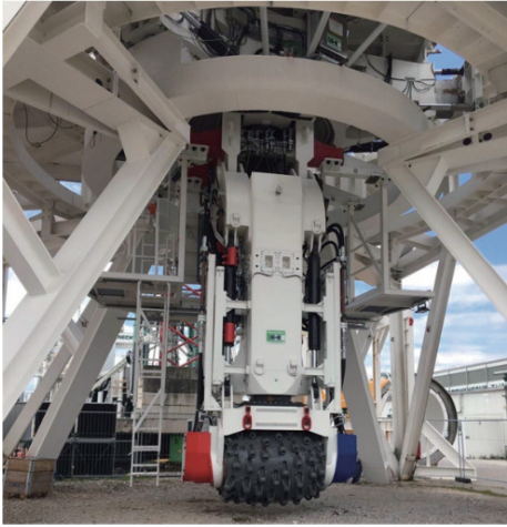
图 11 Woodsmith 项目竖井掘进机 Fig.11 SBR shaft boring machine in Woodsmith potash mine
