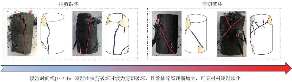
图 6 煤样典型宏观破坏及过渡示意 Fig.6 Typical macroscopic failure and transition diagram of coal sample
