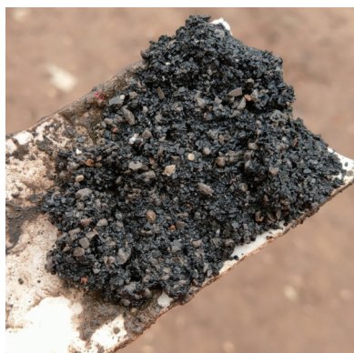
图 3 岩屑出现注浆材料 Fig.3 Presence of grouting material in rock chips
