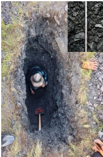
图 9 采坑回填区渣土冻结状况探坑观测 Fig.9 Freezing observation of dregs in backfill area of mining pit
