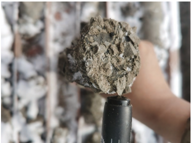
图 10 ZK-5 号钻孔含冰屑岩心照片 Fig.10 Photo of ZK-5 borehole core containing ice debris
