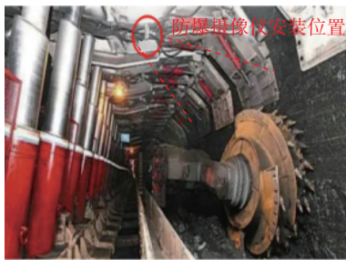
图 1 视觉传感器布置示意 Fig.1 Arrangement method of camera
