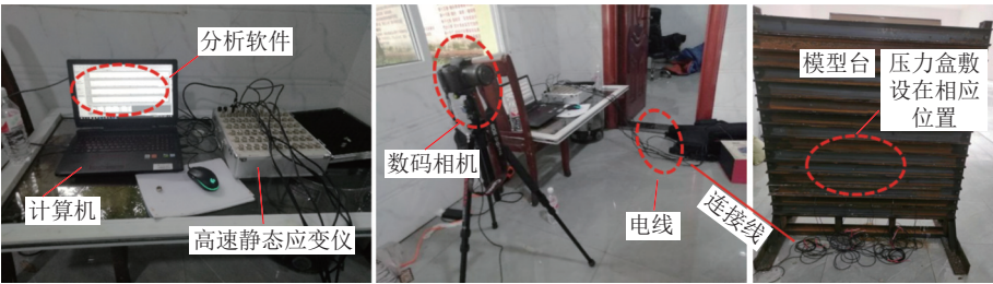
图 12 应变数据采集分析系统 Fig.12 Strain data acquisition and analysis system
