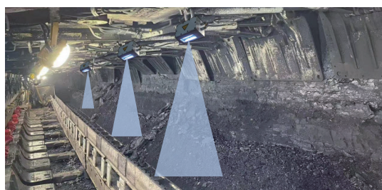
图 8 矿用 3D 摄像机在采煤工作面的安装 Fig.8 Installation of mine 3D camera in coal face
