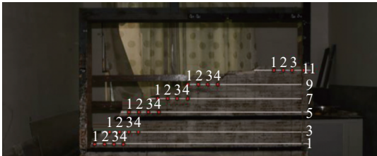
图 7 边坡测点布置 Fig.7 Layout of slope measuring points
